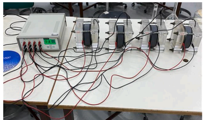
Fig. 7. RCPT instrument used in this study.
