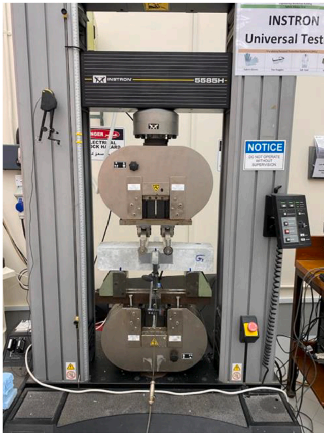
Fig. 5. Flexural tensile strength test setup.
