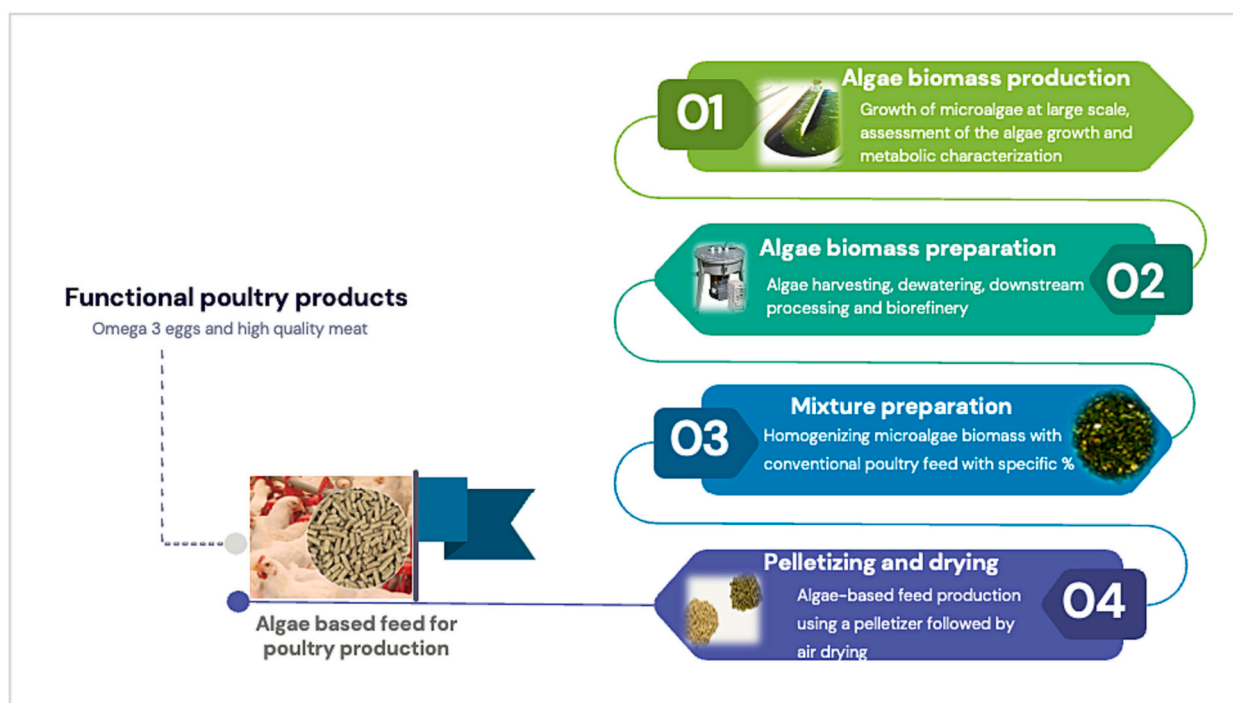
Fig. 2. Process chart of producing functional poultry feed enhanced with microalgal biomass.
