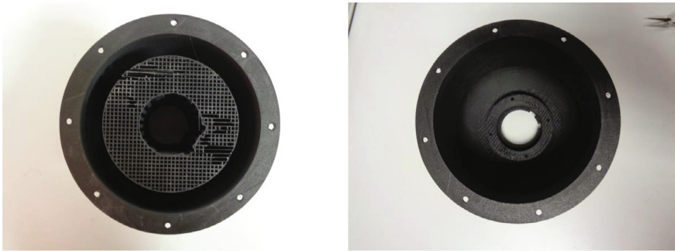
Fig. 8. Before and after the removal of the support material from inside the dome housing.
