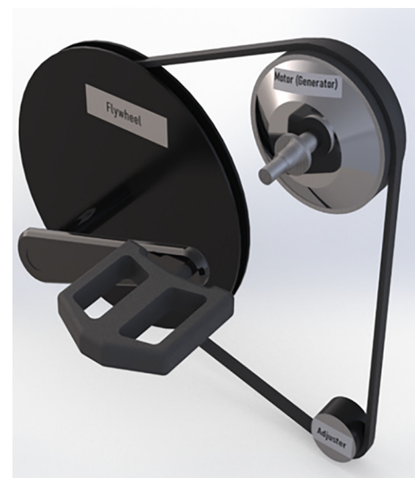
Fig. 5. Dynamo/flywheel connections.
